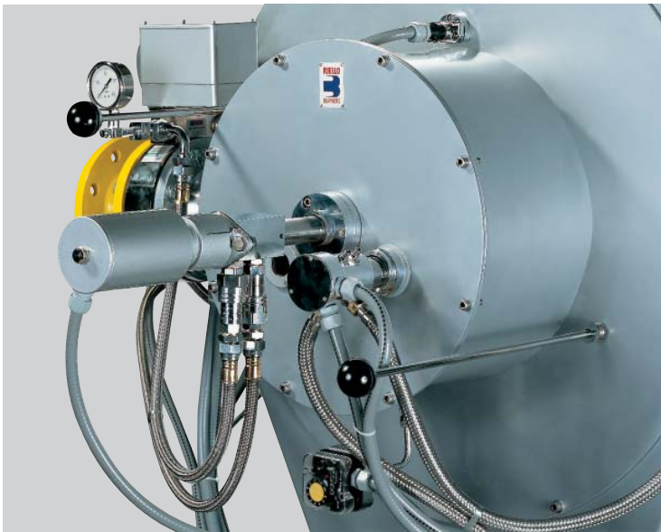
Example of axial swirl register device
